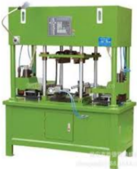
YCL-630B 半自動三模頭 YCL-630B 3 semi-automatic centrifugal casting machine with three mould
